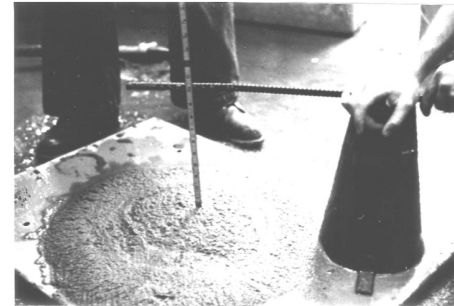
(a) Slump Test of Fluid Grout
