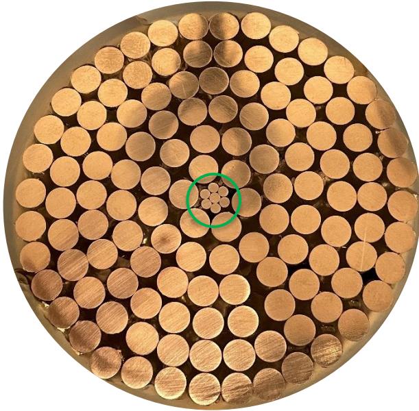
Cross section of 3 1/4-inch diam. M4N AUX cable
