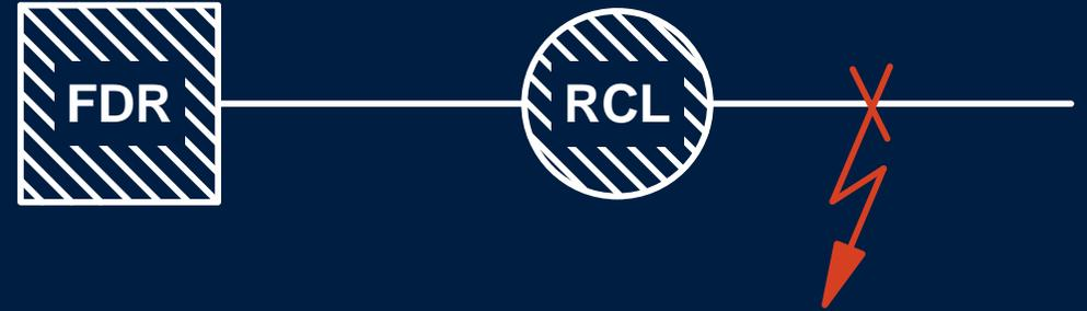
Magnetic field from fault current causes upstream conductors to contact
